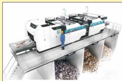
(Fig. Robotic e-waste sorting system. Source: www.nbcnews.com )
