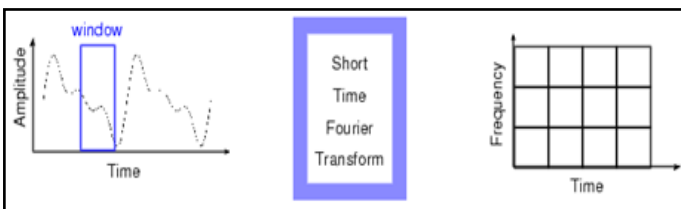
Fig. 3: Basic Principle of STFT [1]
