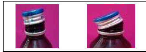
Fig.2 Sample Images of faulty bottle cap from dataset
