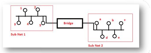
Here in this diagram we see that <u>Sub Net 1</u> and <u>Sub Net 2</u> are connected through a bridge. If the <u>PC 'b'</u> wants to send something to <u>PC '2'</u> the bridge will let the packets move across. Similarly if 'b' wants to send something to 'd', the bridge will not allow packets to move across.
