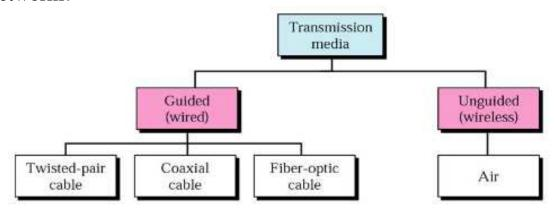
Guided media:- This kind of transmission media is also known as wired otherwise bounded media. In this type, the signals can be transmitted directly & restricted in a thin path through physical links. The main features of guided media mainly include secure, high-speed, and used in small distances.
