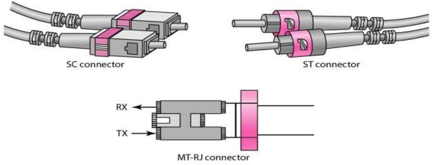
The Subscriber Channel(SC) connector is used for cable TV. It uses push/pull locking system. The Straight-Tip(ST) connector is used for connecting cable to the networking devices. MT-RJ is a connector that is the same size as RJ45.
