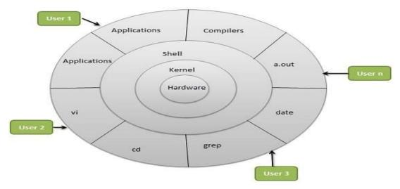
The architecture of a Linux System consists of the following layers -
