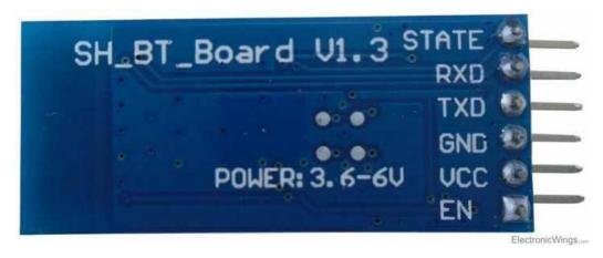
Bluetooth serial modules allow all serial enabled devices to communicate with each other using Bluetooth.
