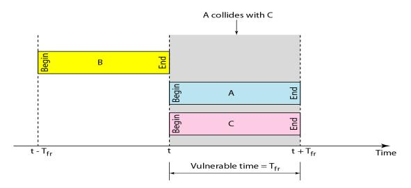
Station A sends a frame at time t. Now imagine station B has already sent a frame between  $t-T_{fr}$  and t. This leads to a collision between the frames from station A and station B. The end of B's frame collides with the beginning of A's frame. On the other hand, suppose that station C sends a frame between t and t +  $T_{fr}$ . Here, there is a collision between frames from station A and station C. The beginning of C's frame collides with the end of A's frame.
