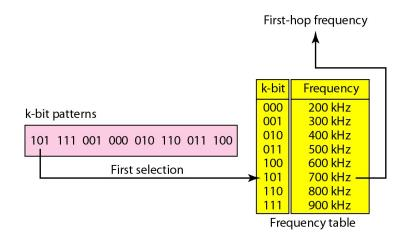
The pattern for this station is 101, 111, 001, 000, 010, 110, 011, 100. The pattern is pseudorandom it is repeated after eight hoppings. This means that at hopping period 1, the pattern is 101. The frequency selected is 700 kHz; the source signal modulates this carrier frequency. The second k-bit pattern selected is 111, which selects the 900-kHz carrier; the eighth pattern is 100, the frequency is 600 kHz. After eight hoppings, the pattern repeats, starting from 101 again.
