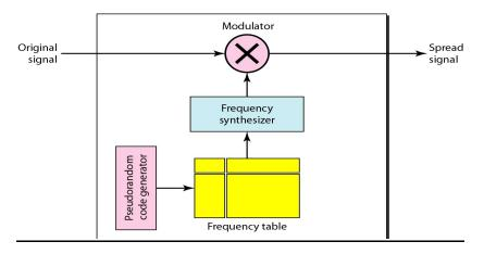
• Suppose we have decided to have eight hopping frequencies. In this case, *M* is 8 and *k* is 3. The pseudorandom code generator will create eight different 3-bit patterns. These are mapped to eight different frequencies in the frequency table.
