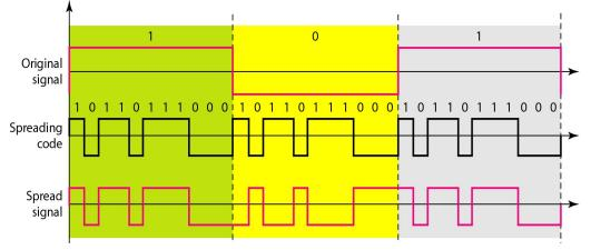
• Thus, this scheme can accomplish the goals of spread spectrum by providing privacy if the intruder does not know the code and also it can provide immunity against interference if each station uses a different code.
