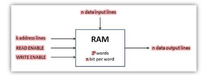
**Write Operation to RAM:** Write operation in a RAM is accomplished by the following steps:
