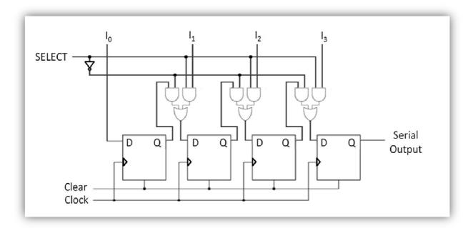
Here as we see in this diagram, first flip-flop gets a fresh input  $(I_0)$ , but the second is given two options- either to get fresh input  $(I_2)$  or to get output (Q) of previous flip-flop. This is literally what we call parallel input but serial output.
