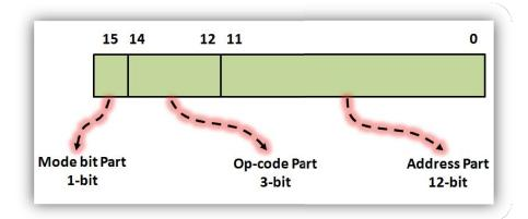
The proposed instruction format and its parts are based on a 16-bit register size.
