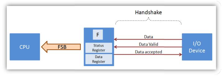
**Interrupt Driven I/O:** Interrupt driven I/O is a little complex because an I/O instruction suddenly intervenes the CPU in such a way that it has to pause its running task and process the I/O instruction. After processing it, CPU returns to the paused task.
