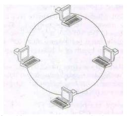
Computers connected in a ring or circular topology Performance on this type of topology is faster because each portion of the cabling system handles only the data
