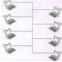
computers attached to a bus network can significantly affect the speed of the network. A computer must wait until the bus is free before it can transmit. Each node is connected to two others except the machines at either end of the cable, which are connected only to one other node. Ethernet 10Base2 (also known as thin net) is an inexpensive network based on the bus topology.
