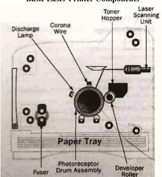
**Basic Laser Printer Components**
