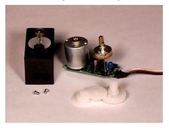
Working of a Servo Motor
