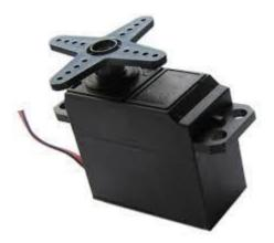
Servos are extremely useful in robotics. The motors are small, have built-in control circuitry, and are extremely powerful for their size. A standard servo such as the Futaba S-148 has 42 oz/inches of torque, which is strong for its size. It also draws power proportional to the mechanical load. A lightly loaded servo, therefore, does not consume much energy.
