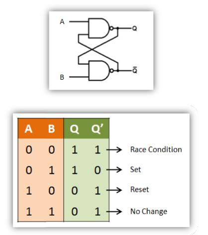
**Flip-Flop:** A Flip-Flop is a basic electronic circuit that is designed to store a single bit either it is a "0" or a "1". Thus we can say that a Flip-Flop is the smallest unit of an Electronic Memory.
